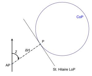
The Marq St. Hilaire – Altitude intercept method in Celestial Navigation, use the tangent line to the circle of equal altitude close to the estimated position of the observer.
