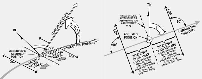
Figure 11.2. Line of Position Computed by Intercept Method.
