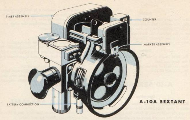
Determine the number of impulses of the marking mechanism per minute. Normally this number does not vary greatly even with extreme changes in temperature. Once you know it, you need only to count the clicks of the solenoid to time an observation.
