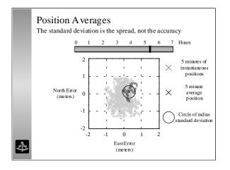
Here is a 5-minute occupation that has a standard deviation about equal to the accuracy of the 5-minute average position.
