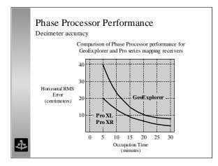
Now we can compare the Phase Processor performance of the GeoExplorer and the Pro XL/XR receivers. At all occupation times the Pro XL/XR receivers provide twice the accuracy of the GeoExplorer. For all receivers, longer occupation times improve accuracy. Decimeter accuracy is achieved after ~15 minutes for the Pro XL/XR and after ~22 minutes with the GeoExplorer.
