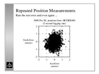
Base receiver: Pro XL with firmware version 3.08 Rover receiver: Pro XL with firmware version 3.08
