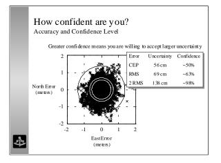
have very small errors and others have errors as large as 1.5 meters, or more. With this kind of plot it is very difficult to say very much about the accuracy. So many of the positions are overlapping each other it is difficult to see how many are near the origin - the true position of our test site. A better way to view these data is with a histogram of the horizontal error.
