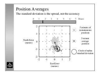
Be careful to note here that the standard deviation is much smaller during this 5 minute occupation than the average position's accuracy (distance from the origin).
