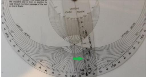
**Figure 4:** Setting the Declination onto the Latitude, the green arrow shows the intersection of the declination and the latitude. Note the green arrow is not present on the physical device. With all the settings made, we can see the words "TIME OF SUNSET" and the cursor directly on 1740.
