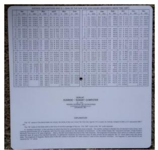
**Figure 1:** Reverse side of the Dunlap Sunrise-Sunset Computer, showing the tabulated values of G and Declination as a function of the day of the year.
