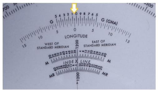
*Figure 2:* Set the circular disk index to the G value given for the date. The white/ yellow arrow is added for emphasis, so that the reader can see this setting. It is not present on the actual device.
