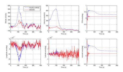
Figure 2. State estimation errors: Modified MMAE-and MMARE- based radio beacons/IMU integrated navigation.
