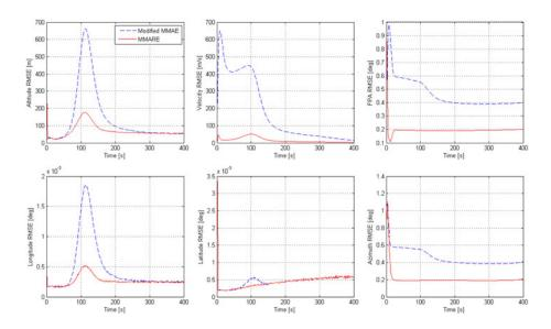
Figure 5. State estimation RMSE: Modified MMAE-and MMARE- based radio beacons/IMU integrated navigation.
