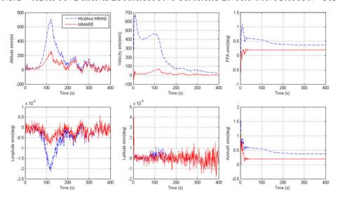
Figure 4. State estimation errors: Modified MMAE-and MMARE- based radio beacons/IMU integrated navigation.
