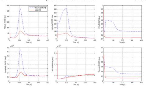
Figure 3. State estimation RMSE: Modified MMAE-and MMARE- based radio beacons/IMU integrated navigation.
