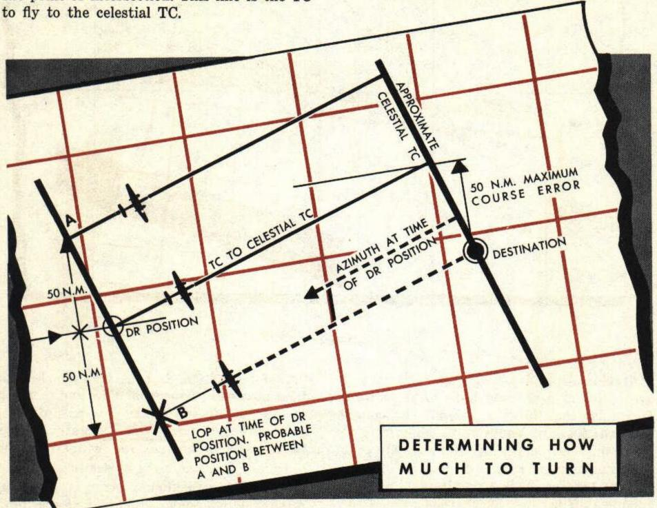
constructed to the celestial TC. Since your estimate of the maximum error at destination included an allowance for DR error on this leg, you should strike the course line on the correct side of destination.
