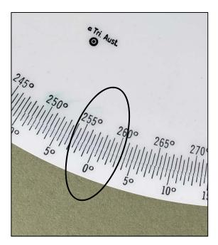
4. Align the observer's Meridian Arrow to the anticipated DR longitude at twilight. Use the rotation arm to rotate the altitude/azimuth disk so that the observer's Meridian Arrow points to the anticipated DR longitude on the outer longitude wheel. West longitudes are clockwise rotations from 0°, east is counter clockwise. A reminder of east/west rotation directions is printed on the star base. In this
