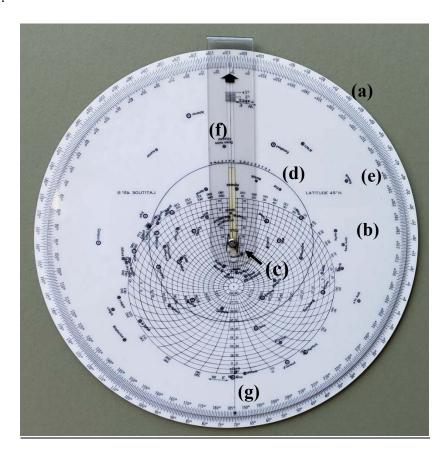
Full view of the CP-300/U USAF Star Finder. Star base is northern hemisphere side (indicated by a large "N" in the center). The altitude/azimuth disk overlay is for latitude 45°N. The disk latitude has been adjusted -5° to more closely approximate the vessel's DR latitude of 40°N. The disk's GHA Aries is set for 257°, the expected hour angle for twilight. The viewer's DR longitude is set for 70° West. These adjustments are explained step-by-step below and used in the sample problem.
