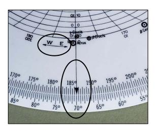
example problem, the meridian pointer is set to 70°W longitude. Note that once the altitude/azimuth disk is oriented, LHA of Aries 187° can be read above the DR longitude. This step is the similar to the 2102-D however the navigator only has to work with his DR longitude and GHA of Aries. LHA of Aries is simply the DR longitude offset to Aries.
