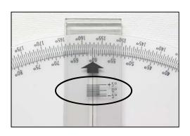
O Below the horizon altitude scales – the CP-300/U overlay disks extend the azimuth grids to -10° below the visible horizon. This is a useful addition for estimating which stars are just entering or leaving Civil and Nautical Twilights.
