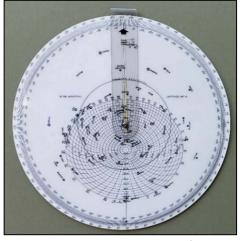
grid projections for north/south latitudes in increments of 10°. Both the 2102-D and CP-300/U use the polar azimuthal equidistant projection of the stars and the oblique azimuthal equidistant projection of the horizon system for the altitude/azimuth disks. See Appendix C for a technical description of these two projections. Note that stars are the mirror image as they appear in the sky like an old-fashioned star globe; you can't hold it up to the sky and use it like a planisphere.
