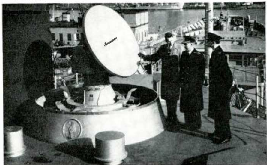
Antenna system of the AN/SRN-4 radio sextant installed on the USS "Compass Island."
