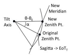
The distance between the original zenith point and the meridian associated with the new zenith point is just the sagitta of the chord formed by new meridian. If we were dealing with planar geometry the sagitta would be given by the radius of the circle times (1–cos  $\alpha$ ). However, in this case we need to use spherical geometry for the solution. Using Napier's Rules<sup>1</sup> for right spherical triangles we can write:
