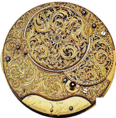
Internal movement of the “K1” timekeeper, a meticulous copy of H4 made by Larcum Kendall and tested on Cook’s second voyage. 1766–69. NMM.
