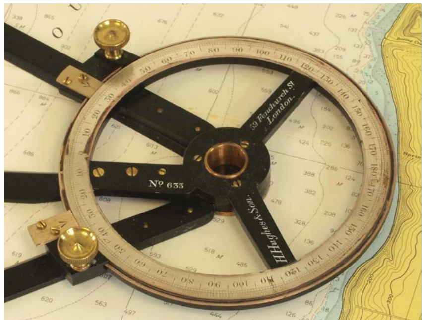
Figure 3. Station Pointer's Scale
