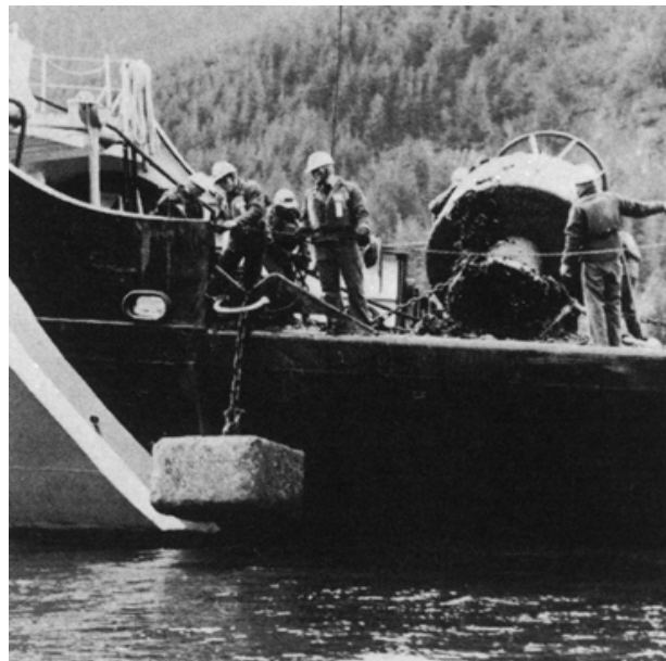
Figure 512. A sinker used to anchor a buoy.
