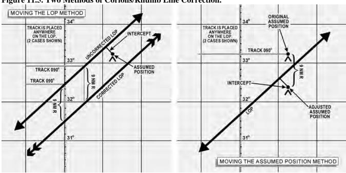
Figure 11.5. Two Methods of Coriolis/Rhumb Line Correction.
