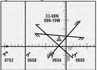
Figure 12.5. Plotting Three LHA.
