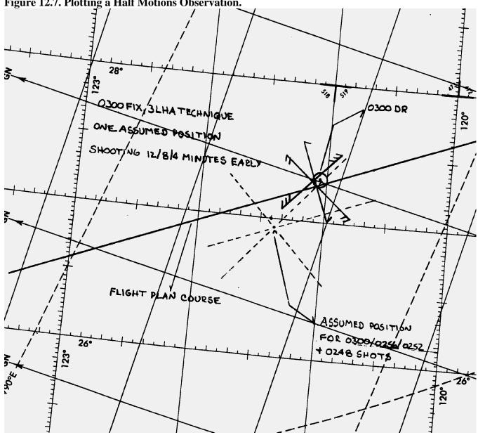
Figure 12.7. Plotting a Half Motions Observation.
