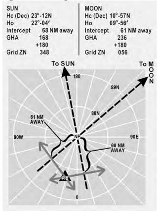
Figure 12.15. Using Pole as Assumed Position.
