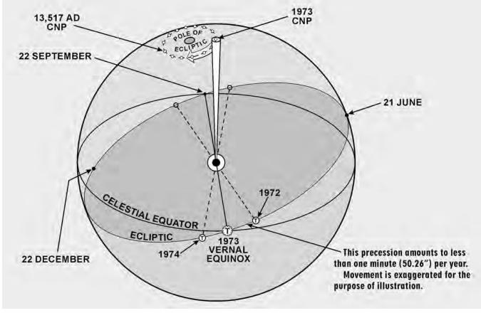
9.13.1. In Figure 9.11, you can see that if the stars remain fixed and the equinoctial moves up and down, the Dec of these bodies is changing.
