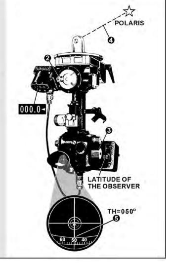
Figure 12.14. Inverse Relative Bearing Method.
