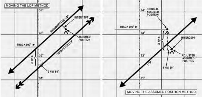
Figure 11.6. Two Methods of Coriolis/Rhumb Line and Precession/Nutation Correction.
