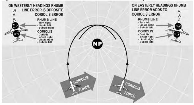
Figure 13.10. Coriolis and/or Rhumb Line Errors in the Northern Hemisphere.
