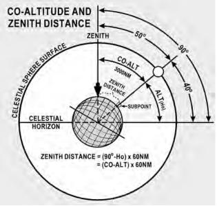
Figure 8.20. Constructing a Circle of Equal Altitude.
