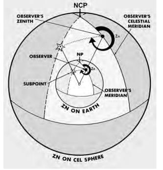
Figure 8.21. Relationship of True Azimuth to an Observer.
