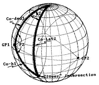
Fig. 7-Navigational Triangle for "Lower" Intersection
