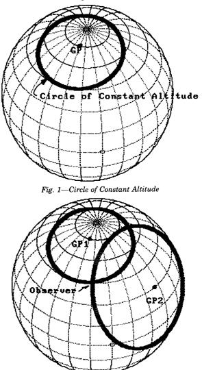
Fig. 2—Two Circles of Constant Altitude Intersecting for a Fix
