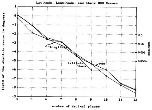
Fig. 8-Error Versus Number of Decimal Places Used in the Calculations
