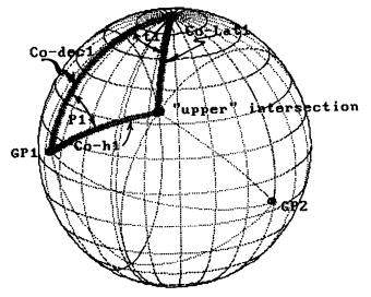
Fig. 6-Navigational Triangle for "Upper" Intersection
