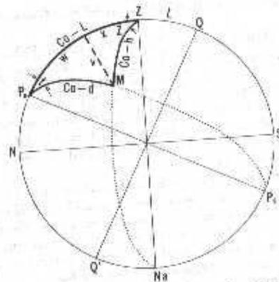
FIGURE 2111.—Navigational triangle with perpendicular from celestial body to celestial meridian.
