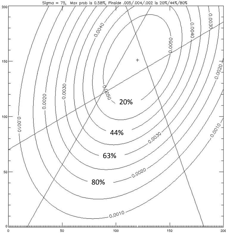
The bold percentages on the contours are the probability that the fix is inside those contours. This is a relatively good fix, with the hat being well within the the individual LOP's standard deviation of 75 units. The "cross" marks the MPP.
