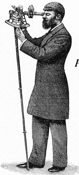
"HEZZANITH" ARTIFICIAL HORIZON, With Night Lamp, and held on Telescopic Stand.
