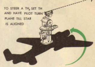
Check heading with astro-compass at intervals of not more than 15 minutes, altering the heading steered on the gyro if necessary.
