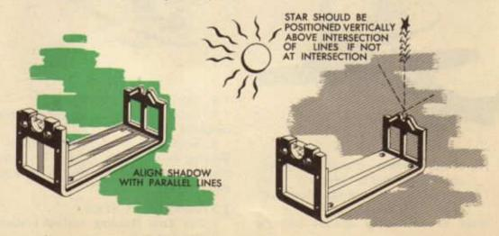
In all uses the astro-compass must be carefully leveled and paralleled with the longitudinal axis. The remaining procedure follows as indicated below:
