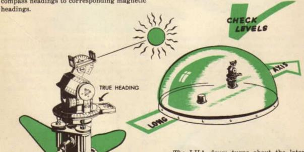
The LHA drum turns about the lateral axis. A dial expressing latitude is connected to a micrometer as well as the drum. The instrument may be used in both hemispheres by following the directions. White numerals are used in north latitudes, and red numerals are used in south latitudes; the 90 is in white only. The knob for setting LHA is opposite the latitude dial. This drum provides a horizon for the instrument.
