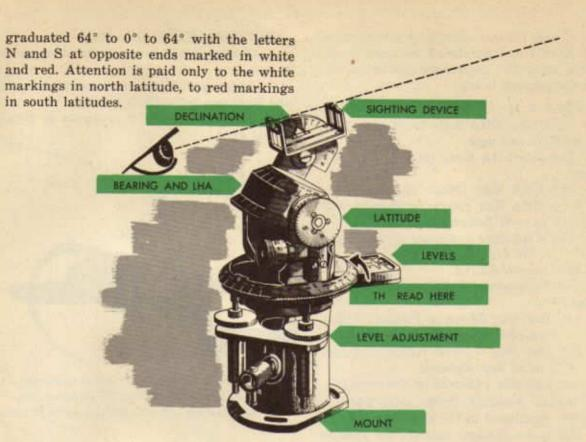
The sighting device is attached to the declination scale bracket. The fore sight is constructed with a shadow bar in the lower area and luminized sight lines at the top. The rear sight is equipped with a lens whose focus is infinity with the fore sight when an object is sighted beyond the fore sight. The rear sight has a translucent screen with two parallel lines to correspond with the fore sight bar. When all settings are accurately made, the
