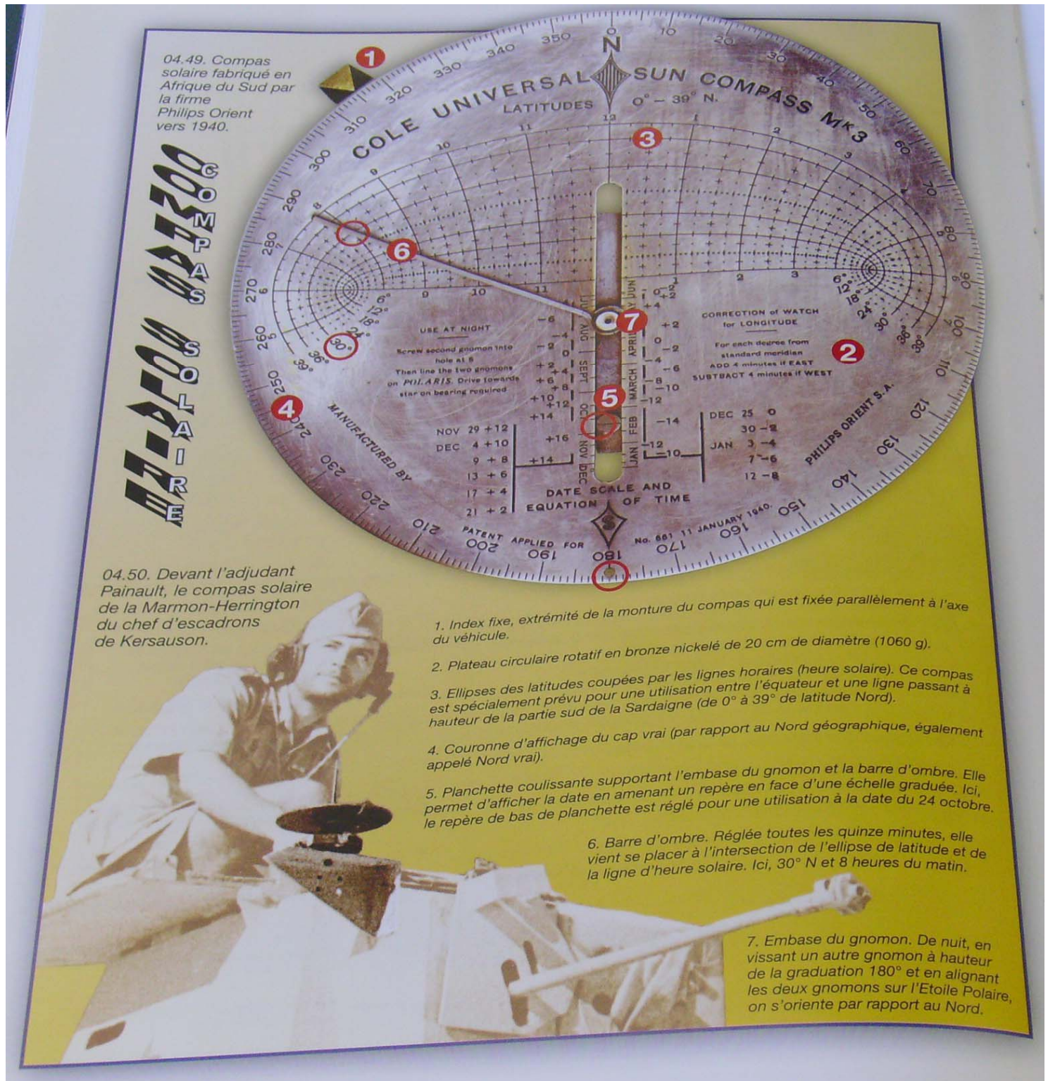
Fig4. The Cole Mk 3 compass in French Army use on a South African made Marmon Herrington armoured car. North Africa, early 1943. After Thierry & Mary Monet.
