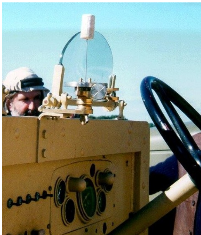
Fig 7. The Bagnold Sun Compass on a Canadian made ‘Chevy’ truck. Note adjusting wheel. Courtesy of the LRDG web site.
