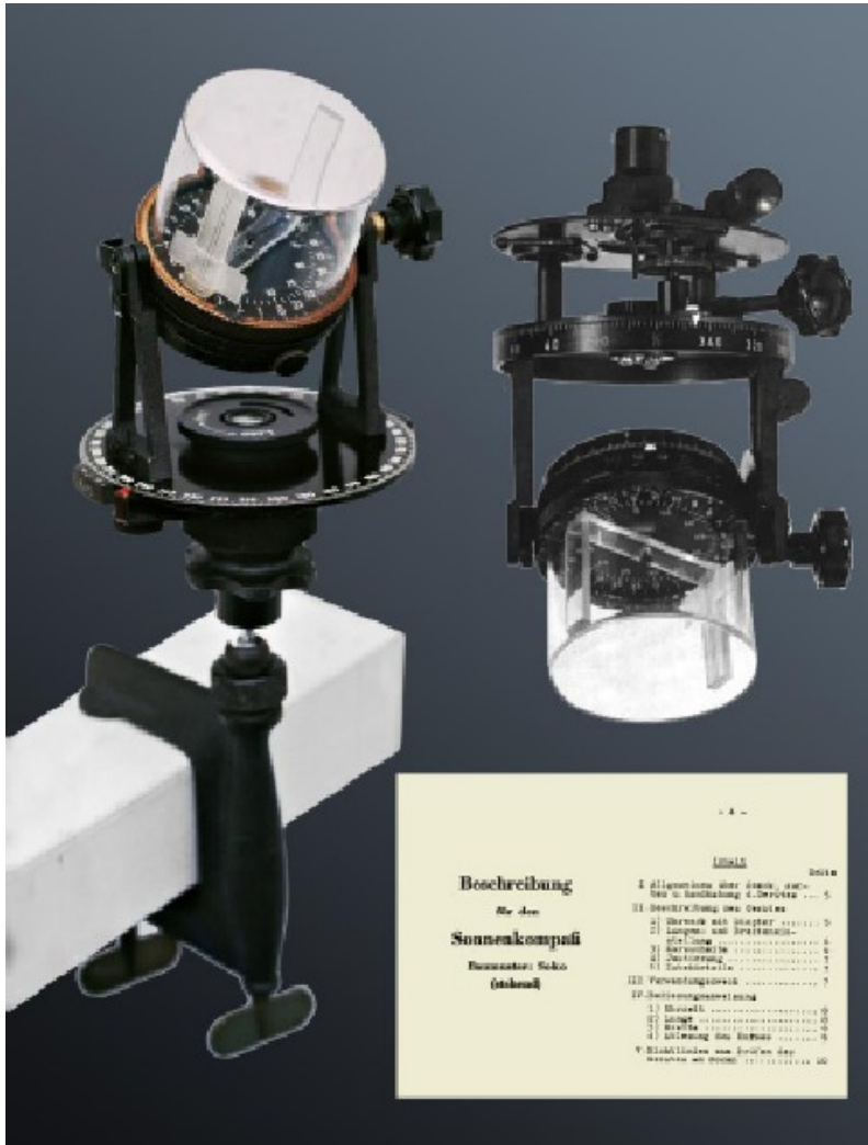
Fig 14. The C Plath of Hamburg Sun Compass. Note sights. Photo by Konrad Knirim
