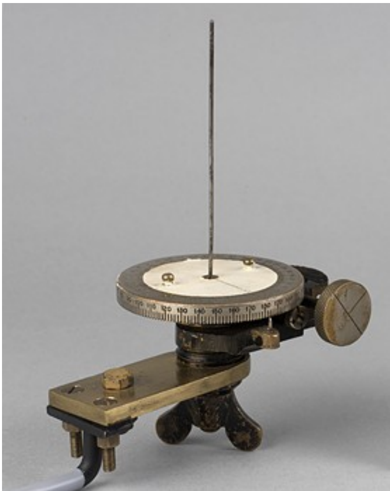
Fig 6. The Bagnold Sun Compass. Photo courtesy of the Imperial War Museum, London.
