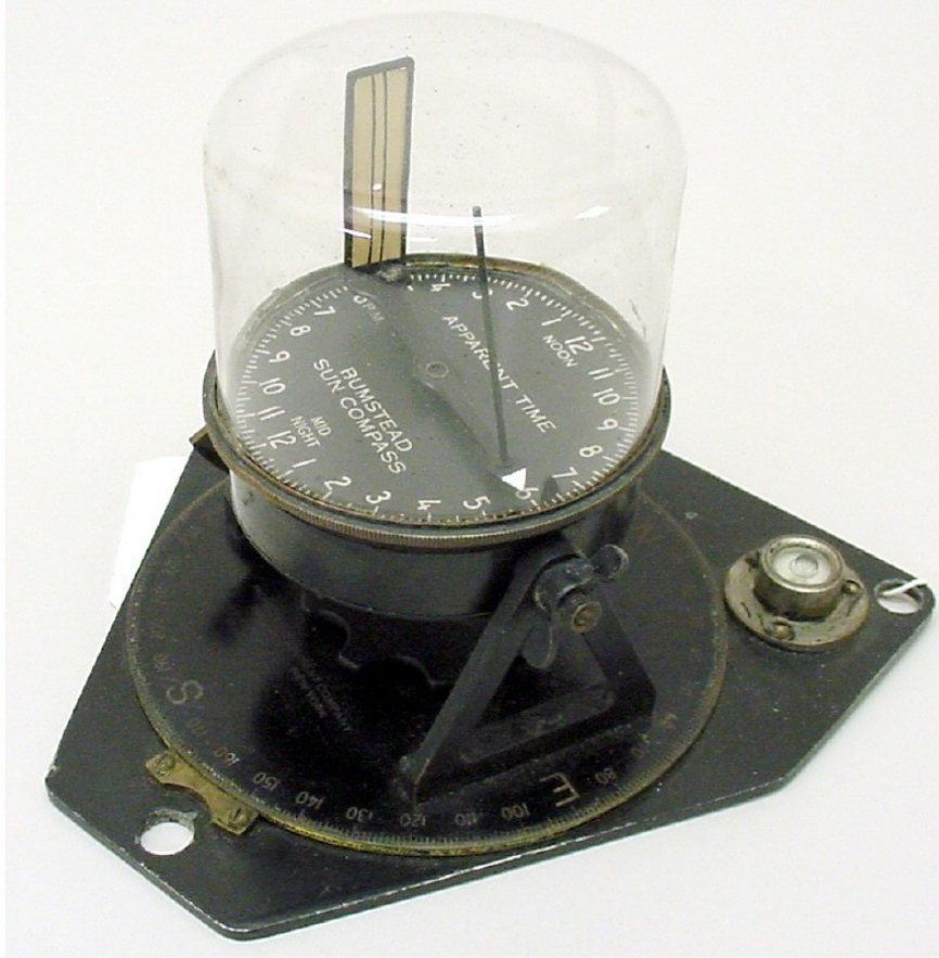
Fig 16. The Bumstead Sun Compass. Note sights. Photo courtesy of the Smithsonian Institute.
