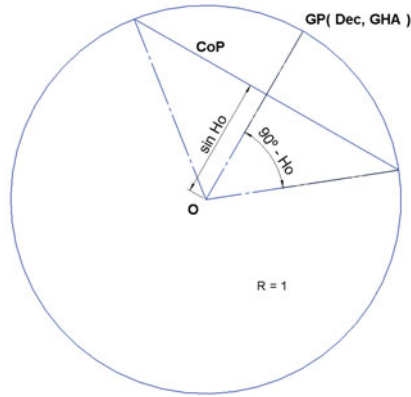
Figure 2. Earth's normal section to the plane of the Circle of Position (CoP).
