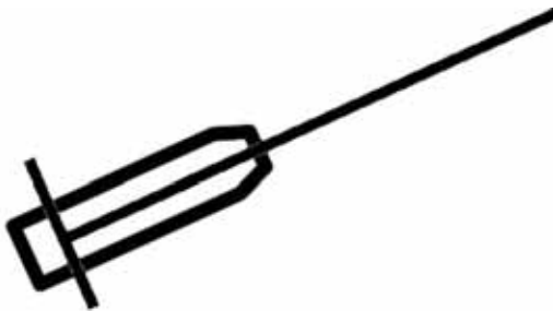
Figure 521b. Example of Own Ship True scale outline (symbol) oriented along own ship's heading. From IMO SN.1/Circ. 243/Rev.1 adapted with permission.
