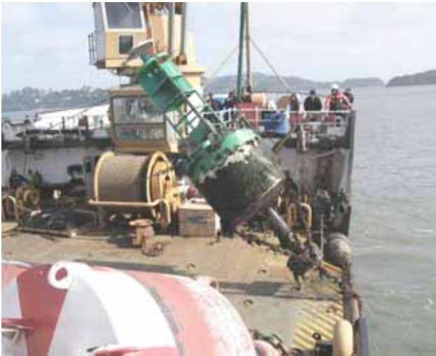
Figure 701a. Buoy with counterweight showing.
