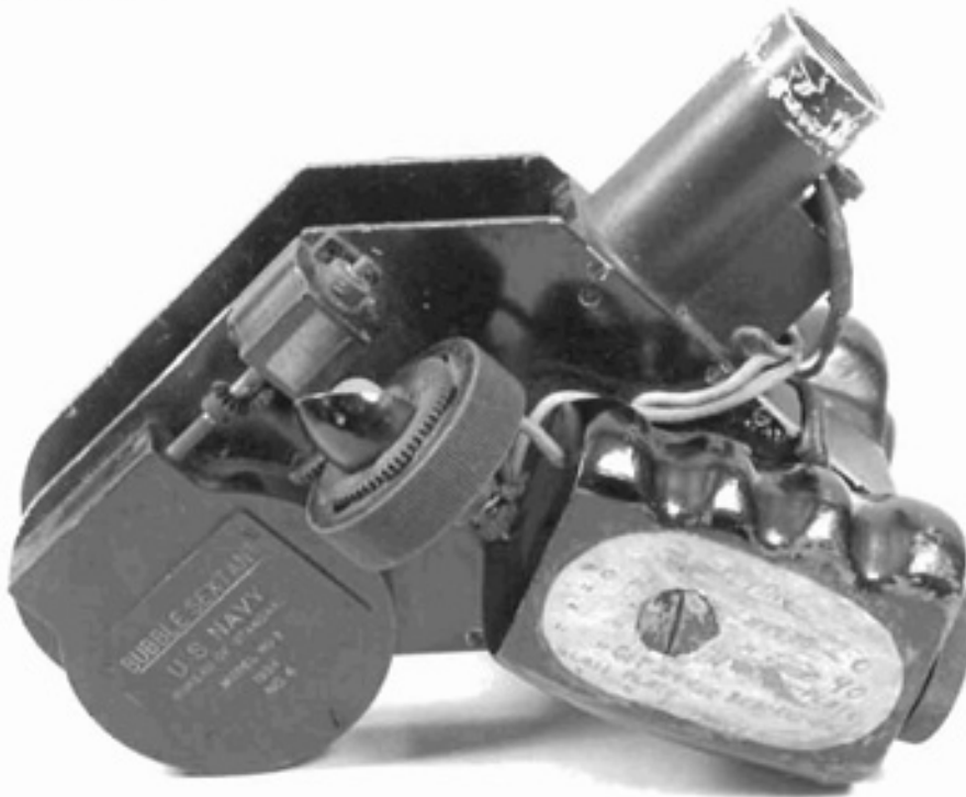
Figure 2 This bubble sextant was developed for the Navy by the Aeronautical Instrument Section of the National Bureau of Standards in 1924, and produced by the Bausch & Lomb Optical Co. (AF*59069-N). (Smithsonian Institution)
