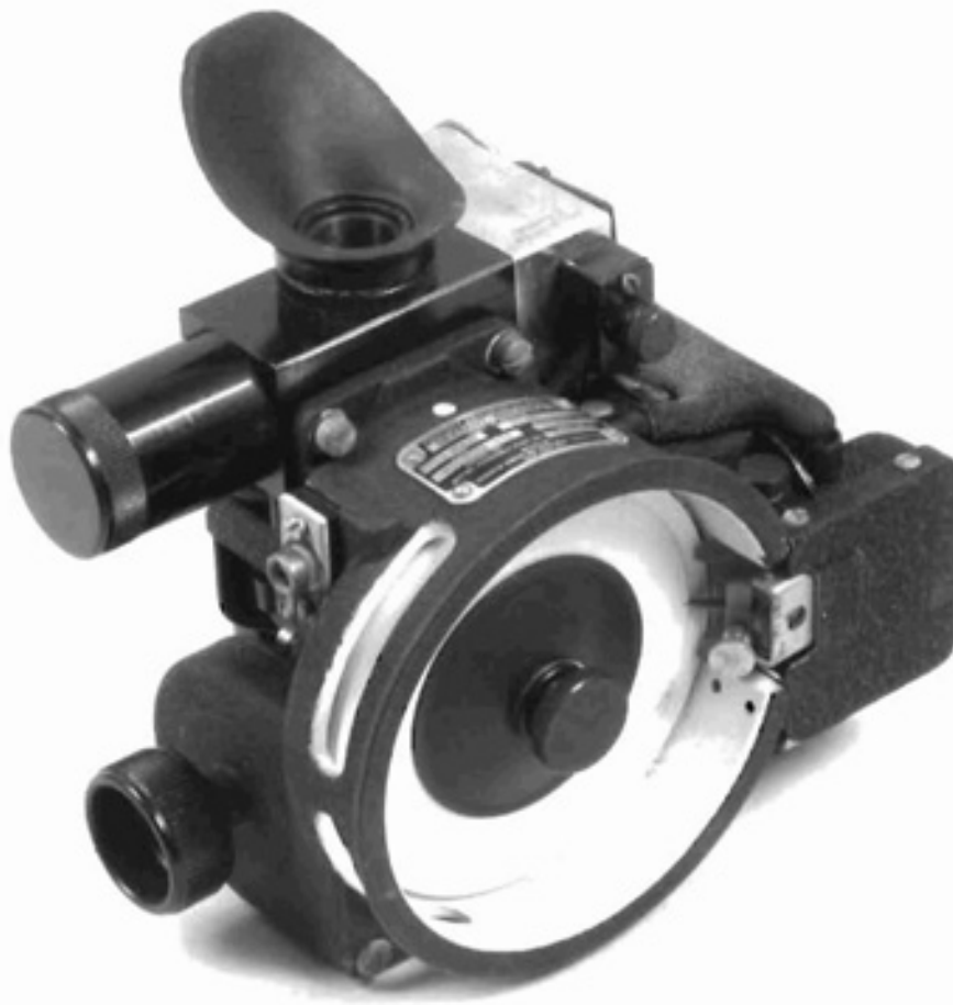
Figure 3 The A-10-A bubble sextant was made for the US Army Air Forces in 1944 by the Fairchild Camera and Instrument Corporation. The navigator would push the plunger while making a shot, thus making a mark on the white plastic disc (AF*59062-N). (Smithsonian Institution)
