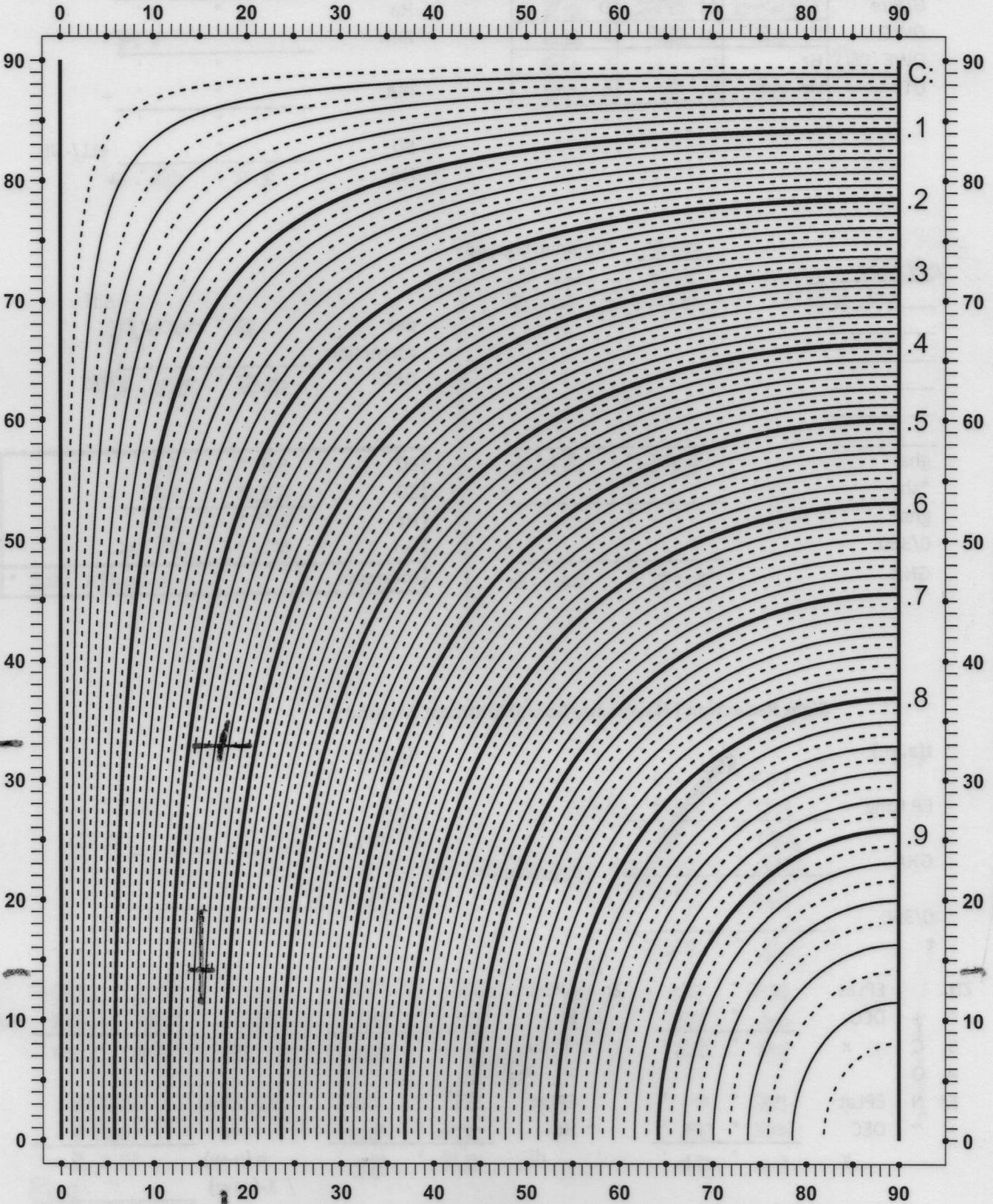
STEP 4: Draw vert. line through pt B. It intersects this axis at pt. Z. Result: AZIMUTH = Z
