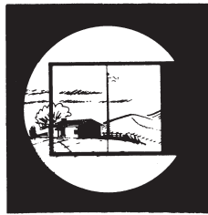
Index mirror screw correctly adjusted.
