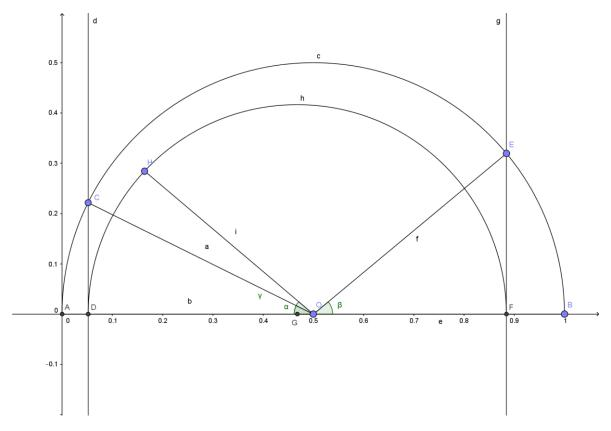
With I being the projection of H on the x-axis and DF being (1 - hav (|B - Dec|) - hav (|B + Dec|), DI becomes (1 - hav (|B - Dec|) - hav (|B + Dec|)) \* hav (LHA) and
