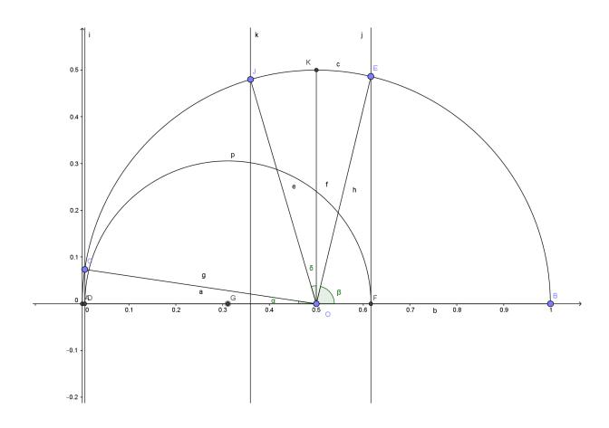
Next define point H at the intersection of the vertical line through J and inner circle DF. Then draw a line GH. The angle DGH (marked  $\gamma$ ) is the azimuth Zn.
