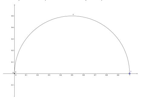
When a line is drawn from the center of the (semi-)circle at angle of  $\alpha$  as the included angle of AOC, the distance AD, with D being the projection of C on the x-axis, is the haversine of  $\alpha$ .
