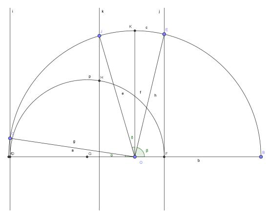
Finally draw a line GH. The angle DGH (marked  $\gamma$ ) is the azimuth Zn. (the angle in between North and the bearing of the sun - or any other heavenly body)
