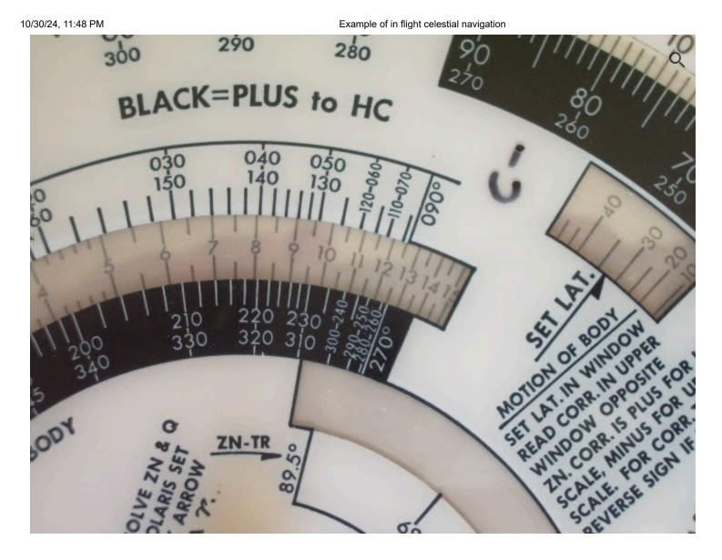
Since all three Zn's are to the west they are all found on the black scale so the signs are all plus. Next, using the relative Zn's (ZN-TR) look in the "CORRECTION FOR MOTION OF THE OBSERVER" window and take out the one minute corrections for MOO (20.jpg , 21.pdf and 22.pdf.)
