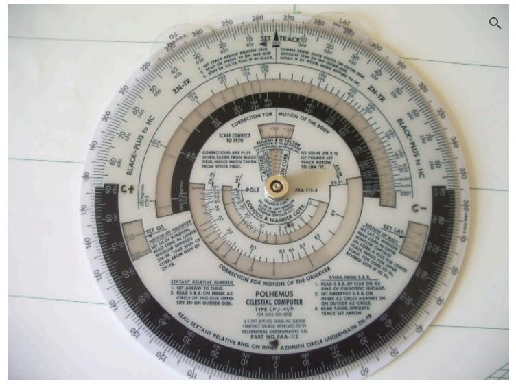
Looking around the outside edge for the Zn's of each body we find the relative Zn's (ZN-TR) and enter them on the form, 75° for Kochab, 15° for Arcturus and 44° for Antares. Using each body's Zn look in the "CORRECTION FOR MOTION OF THE BODY" window and take out the MOB one minute correction and enter it in the appropriate blank (17.jpg , 18.pdf. and 19.pdf.)
