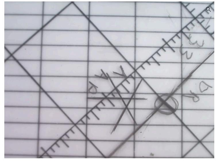
These three lines form the traditional "cocked hat" of a celestial fix. We then move the fix from the center of the cocked hat 1.7 (or 2) NM in direction 356° for Coriolis and then .6 NM in direction 241° for precession and nutation. We do this with visual interpolation since these are small values (30.jpg.)
