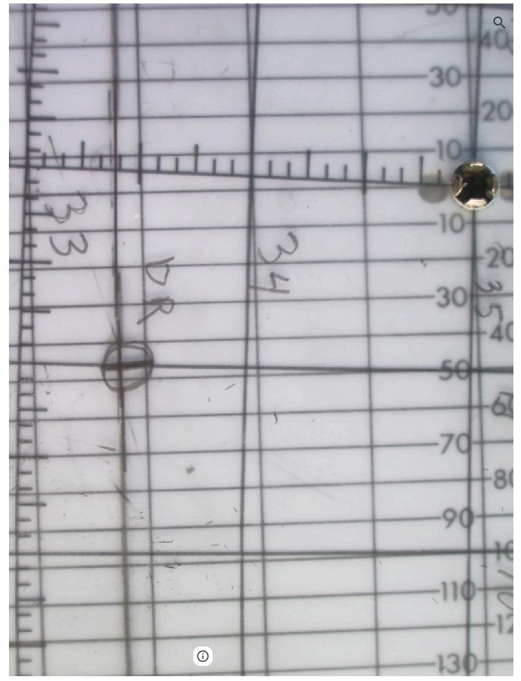
Rotating the grid to north up by placing 360° at the True Index we can read out the coordinates of our 1920Z DR of 33° 27' north,  $11^{\circ}$  00' west (15.jpg.)
