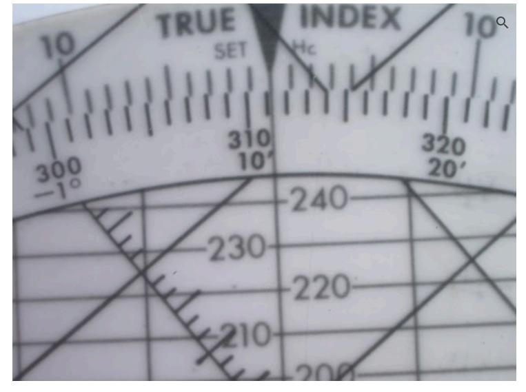
Now we can rotate the disk to place the destination directly above the fix and find the distance and true course to the destination of 284 NM (33.jpg), course 270° (34.jpg.)
