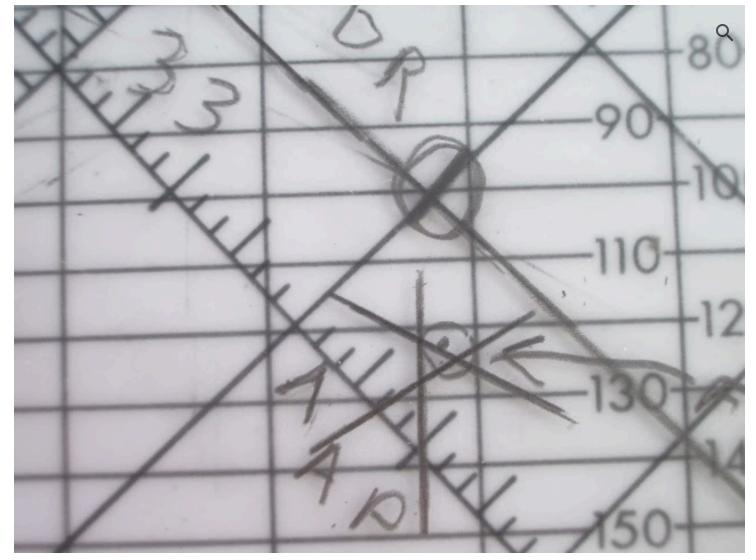
Since the plane flew for 1+14 in cruise we divide this 21 NM by this amount of time and find the wind speed of 17 knots. We now find the direction of true wind as it is already aligned with the "TRUE INDEX" which shows 311° (32.jpg.)
