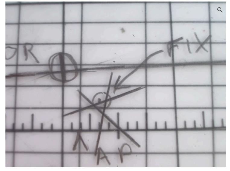
If larger, we would set the respective Zn's under the TRUE INDEX and measure up the appropriate amount for each of these corrections. The fix is 33° 13' north, 10° 41' west.
