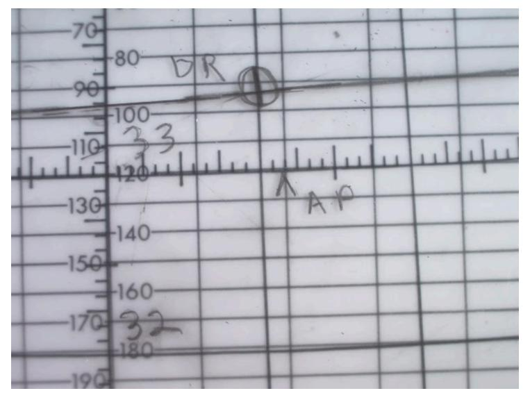
Now set the front of the Polhemus "SET TRACK" pointer to 266°, the "SET GS" (ground speed) to 114 knots and the "SET LAT" to 33° and then tighten the nut to keep the settings from changing (16.jpg.) (We could also do the same adjustments using the MOB and MOO tables from H.O 249.)
