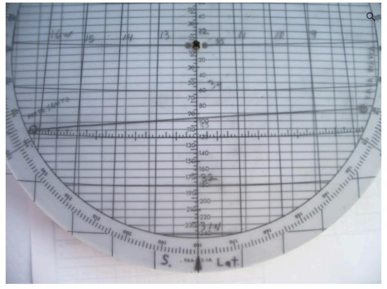
Now, by rotating the disk so that the destination is directly above the departure, we can read out the distance by counting the grid lines between the departure and the destination. Departure is down from the center at minus 215 (visually interpolating between 210 and 220) and destination is up from the center at plus 219 for a total distance of 434 NM (5.jpg.)
