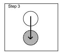
(4) Now turn micrometer Toward you slowly and uniformly so the reflected image rises till the top edge of it just touches the bottom edge of the direct image. And read the dial. It should read something like 32' on the scale -- depending on your IC. Record this ON value. Accurate to the tenth. In this running example we will call this 34.0' ON.
