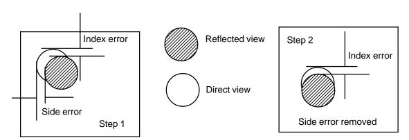
(2) Adjust the side error to remove it by first adjusting the Index mirror to be perpendicular to the frame of the arc and then adjusting the horizon mirror so it is parallel to the frame as well. Then you will see the picture to the right above which is almost all index error with no side error.
