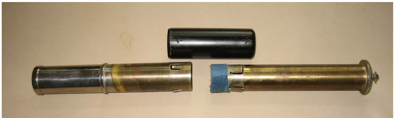
FIGURE 7. Three Parts of an Early Otis King
