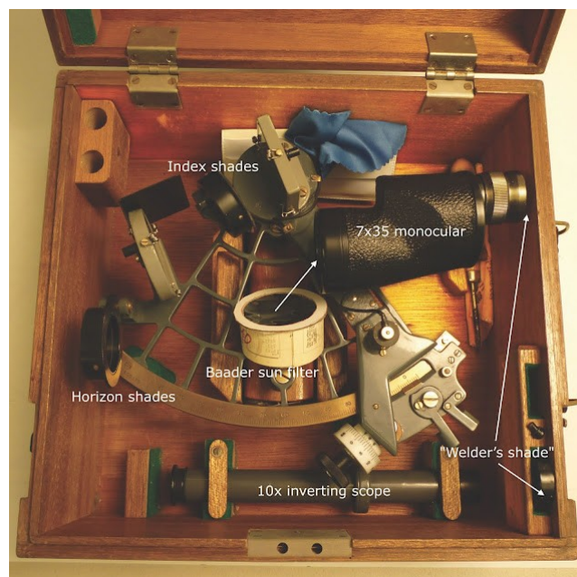
Figure 5. A Tozaki sextant with several features oriented toward the solar IC measurement. The sextant shades are crossed polarized films, which rotate for varied shading.
