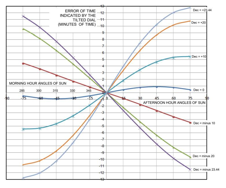
TIME ERRORS IN A SPHERICAL SUNDIAL FROM THE GNOMON BEING INCLINED AT AN ANGLE OF 48.64 DEGREES FROM THE HORIZONTAL ON A DIAL LOCATED AT LATITUDE 41.36 NORTH (ERROR FIGURES OBTAINED FROM SAWYER FORMULA).
