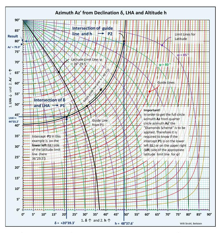
The LHA of the DR-position possibly ranges from 0° to 360°. In the azimuth diagram above however LHA ranges only from 0° to 90° The table below shows which values for LHA' have to be used as entry for the diagram if LHA is outside the range of 0° to 90°.
