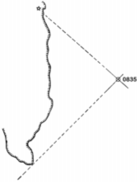
Figure 811a. A fix by two bearing lines.
