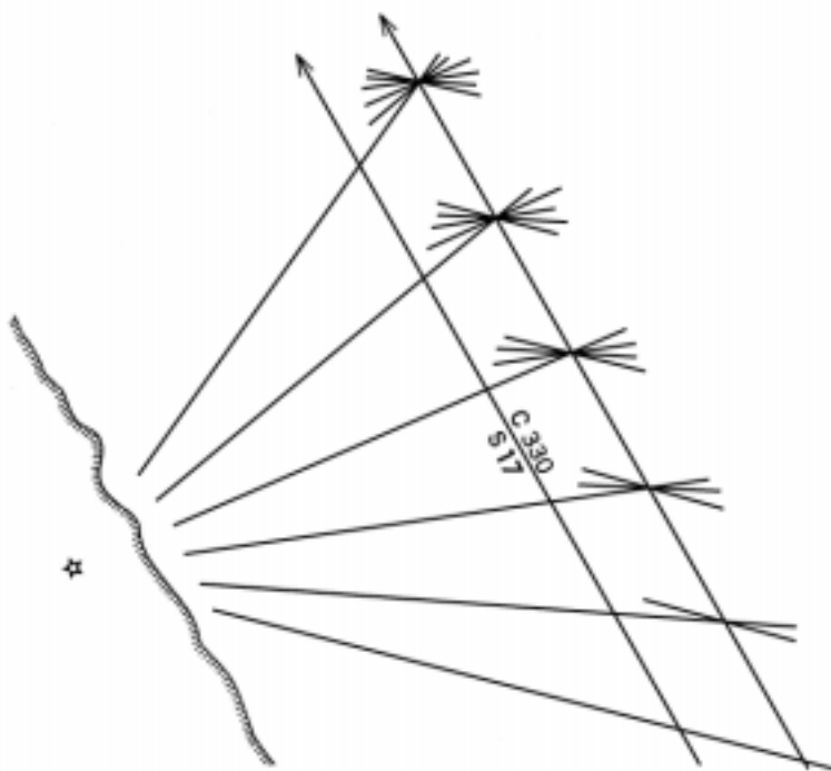
Figure 820b. A number of running fixes with a following current.
