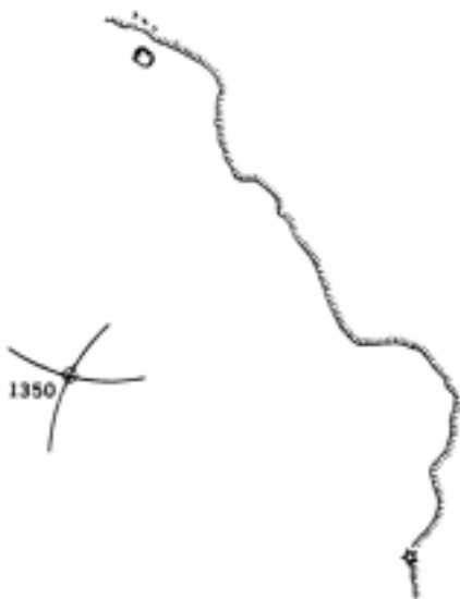
Figure 811b. A fix by two radar ranges.
