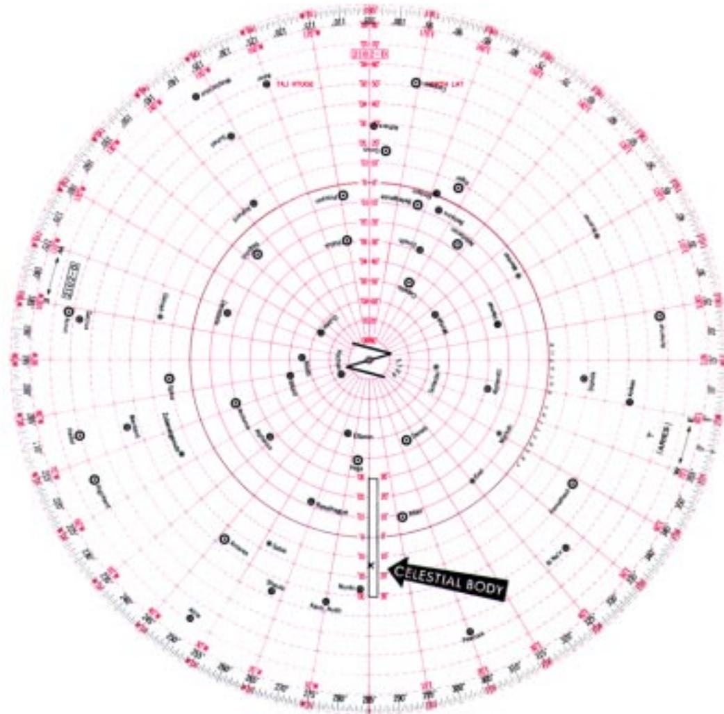
Figure 1539b. Plotting a celestial body on the star base of No. 2102D.
