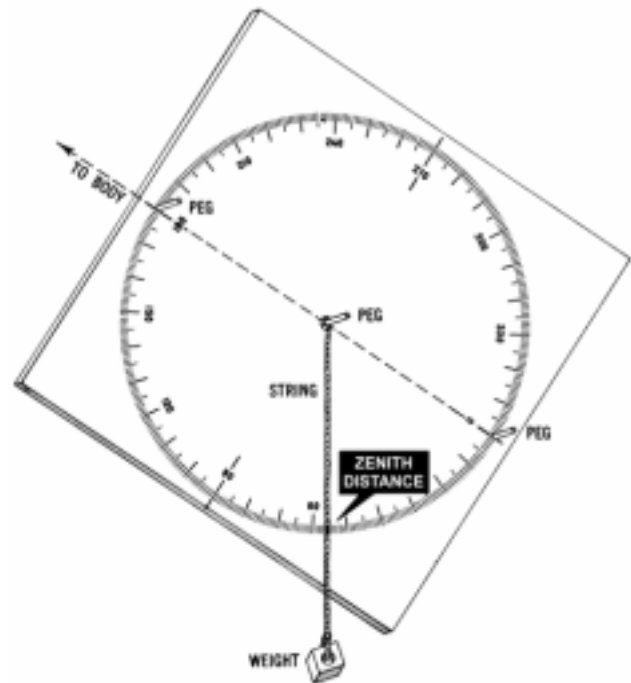
Figure 2608b. Improvised astrolabe; direct sighting method.
