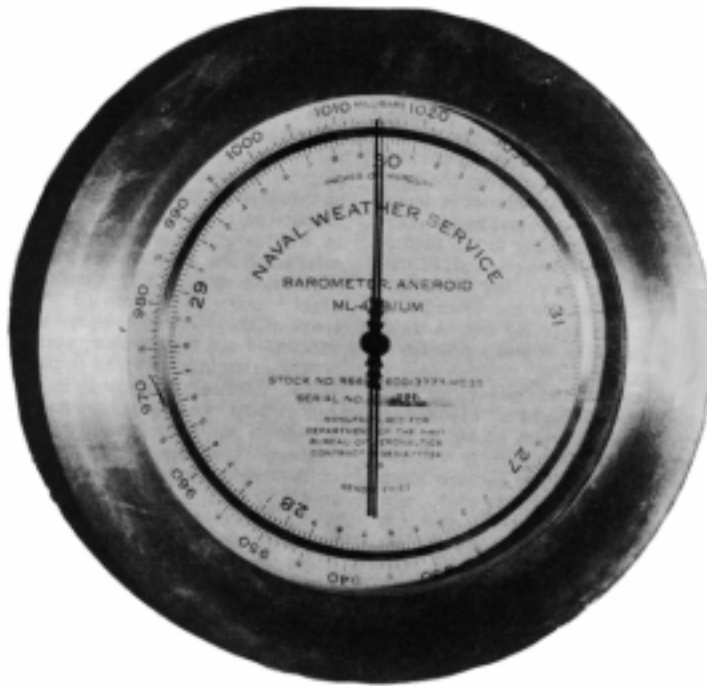
Figure 3703. An aneroid barometer.
